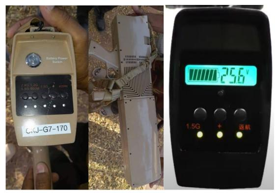
Left: Close-up of the drone jammers, with label marked CKU-G7-170.<sup>132</sup> Right: control panel of CKU jammers, as sold online.<sup>133</sup>
