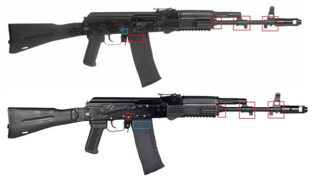
Top image: Saiga-MK 223 Rem.<sup>102</sup> Below: AK-101<sup>103</sup> The Saiga MK has its gas block and front sight pinned to the barrel, as opposed to the AK-101, where they are press-fitted. Additionally, the Saiga-MK lacks an additional rivet immediately above the magazine release catch, and are marked "223 rem" on the magazine.
